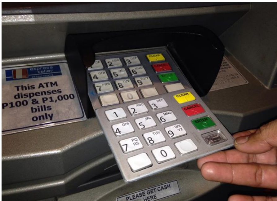
Figure 1.4: The fake keypad on top of the real one logs all the keypresses. This image is taken from [15].
