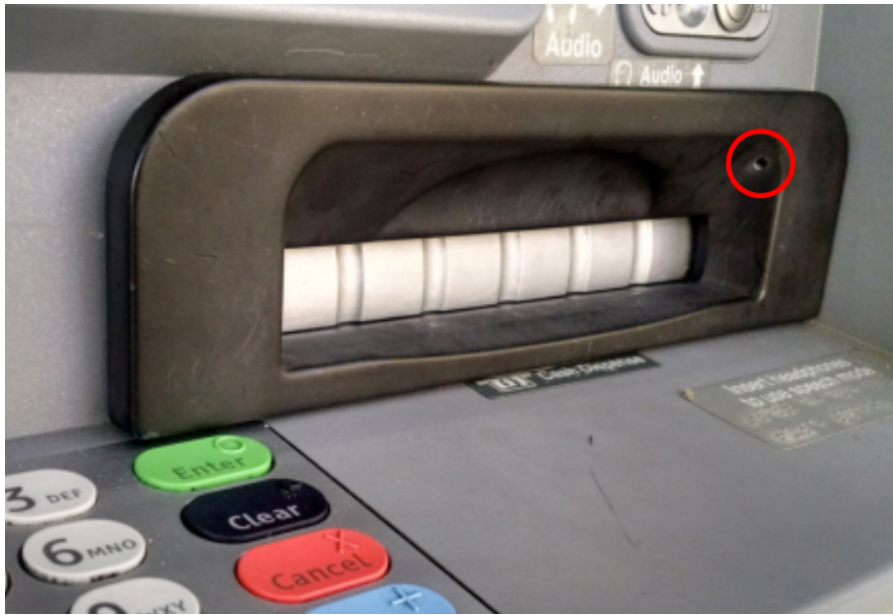
Figure 1.3: The red circle highlights a very small hole from which a pinhole camera was recording the keypad. This image is taken from [15].
