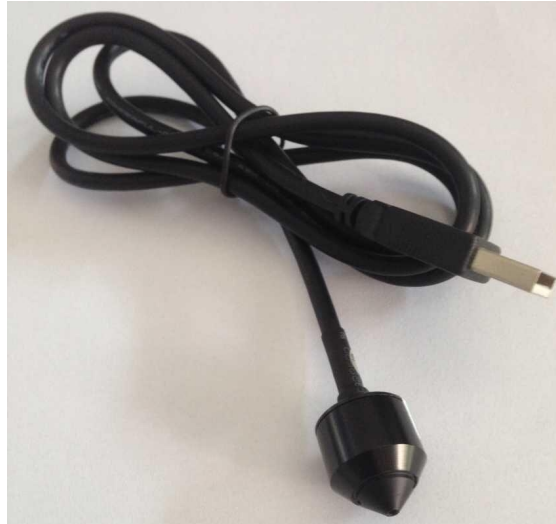
Figure 4.1: Example of a pinhole camera. The camera is usually disassembled to fit in tighter spaces.
