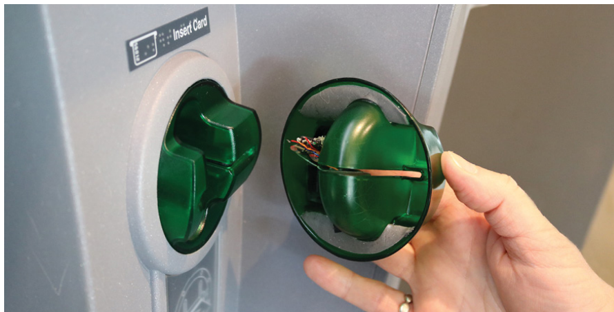
Figure 1.2: The figure shows a fake card tray with a skimmer inside it (the electronic chip). When the fake card tray is put in place, it is not easy to spot unless the victim is very careful to details. This image is taken from [15].
